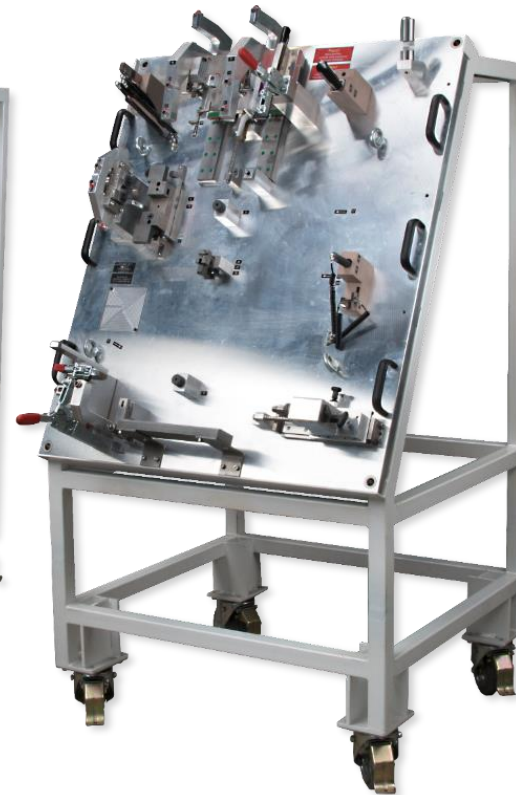
Checking fixtures for automotive seats
