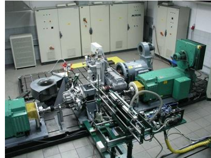
eDrive gearbox testing
