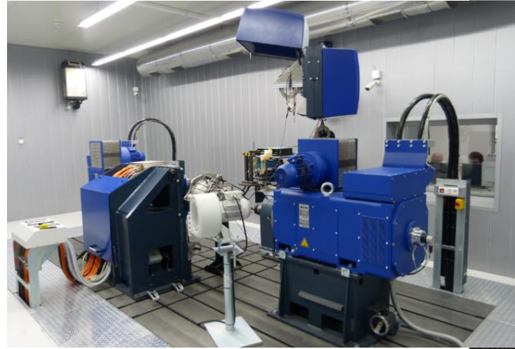
eDrive gearbox testing
