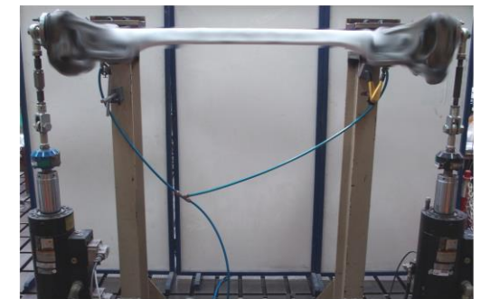
Durability test – multi-axial load
