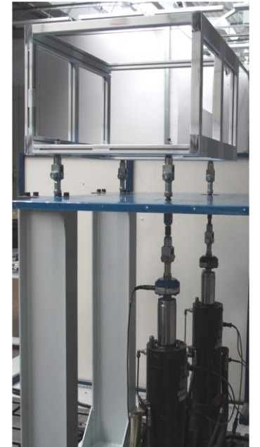
Durability test – multi-axial load
