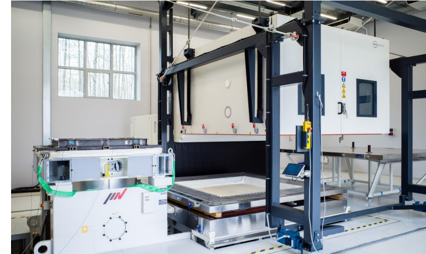
Vibration system dedicated for EV large battery testing
