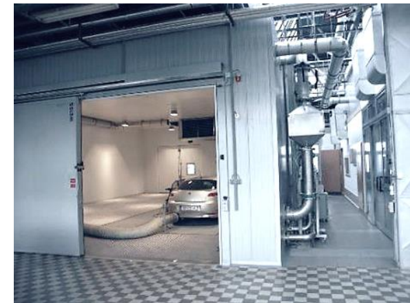
Climatic chamber (-35°C to +60°C) 14,3×10,1×4,3 m
