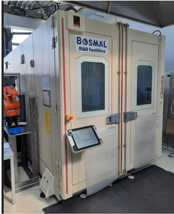
Walk-in climatic chamber 2x2x1.9 m
