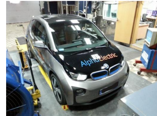
Large dimension climatic chamber Temp.: -45^{\circ}\text{C} - +75^{\circ}\text{C}
